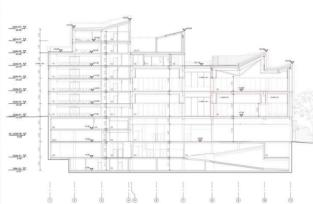
The new MUPAC is divided into two independent above-ground structures that share two common basement levels.
